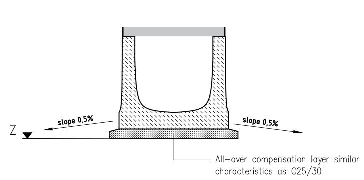
Z =The substructure must be designed long—lasting stable (settlement-free), in order to ensure the transfer of the expected loads without damage.
